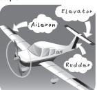
When the plane is in the air, the pilot uses controls to move the plane.
