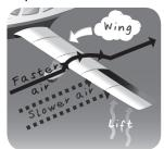
When a plane moves into the wind, its wings cut the wind in half. Some air moves over the plane's wings and some air moves under the wings. The air above the wings moves faster than the air below the wings. This difference in speed makes the plane lift up into the air.
